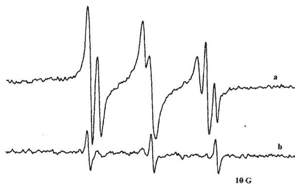
Fig. 4. EPR spectra of PBN adducts obtained after exposure to sun light and left overnight on the system containing riboflavin and collagen a) PBN adducts adsorbed on collagen fibers; b) oxidized or decomposition form of PBN adduct in solution
