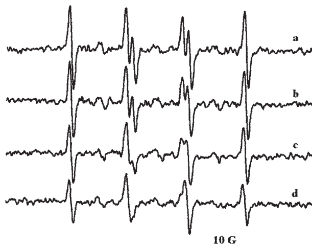
Fig. 6. (a) EPR spectra of DMPO adducts from fresh solution of \text{Na}_2\text{SO}_3 and riboflavin, (b) after 2 min, (c) after 6 min, (d) after 17 min
