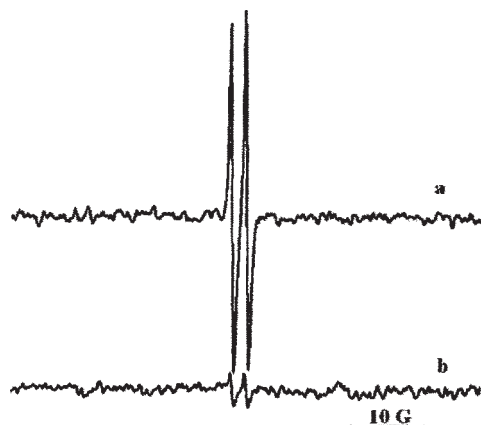
Fig. 5. EPR spectra of ascorbic radical (a) – initial, b) after 20 min
